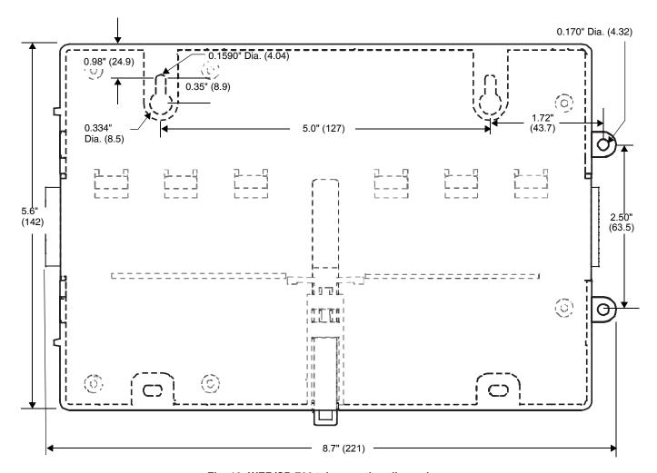
Fig. 13. WEB/CP-700 tab mounting dimensions.
